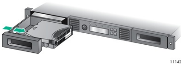
Figure 1. Removing a tape from the mailslot
