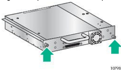
Figure 1. Captive screws on the tape drive
