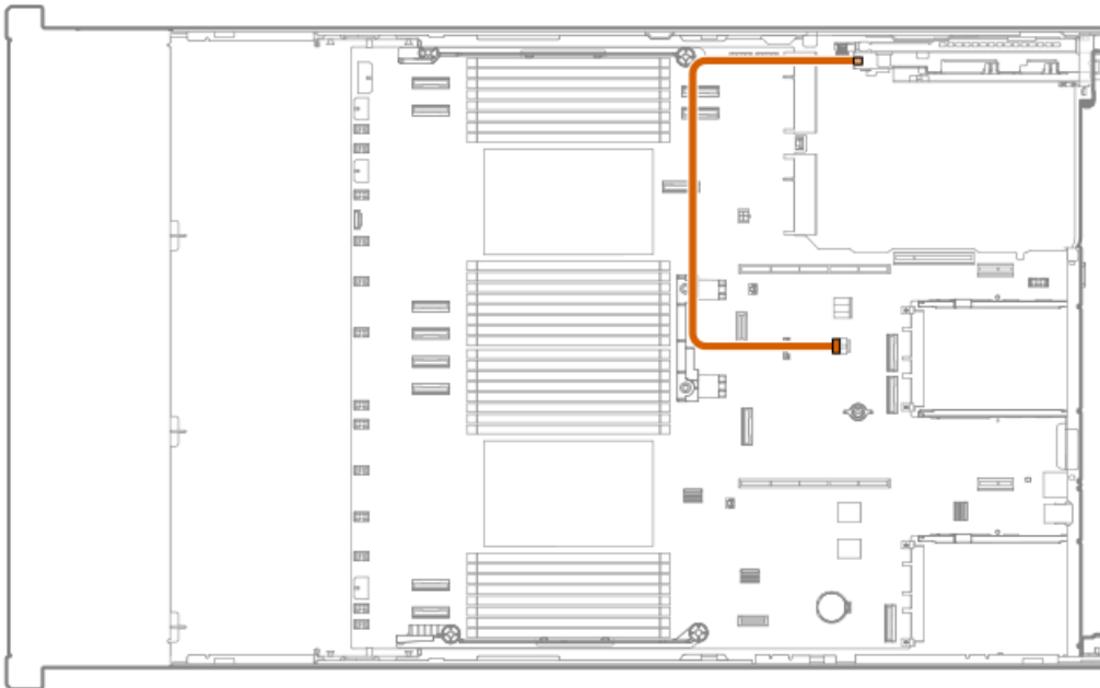
Figure 2. Power cabling for the rear NS204i-u boot device
