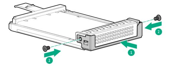
8. Slide the OCP NIC adapter into the E3.S cage until the carrier tab engages with the front OCP NIC bracket.
