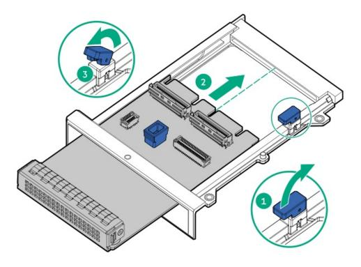
21. If the secondary front OCP NIC adapter is installed, repeat step 21-22 to install the second OCP NIC interposer.
