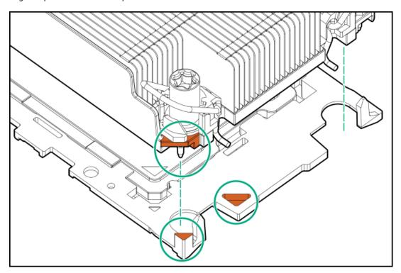
b. Lower the heatsink on the processor carrier until the carrier tabs snap into place.
