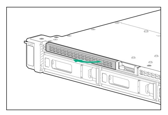
7. Install the optical drive bracket.
