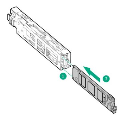
8. Secure the carrier and verify it latches to the device cage.
