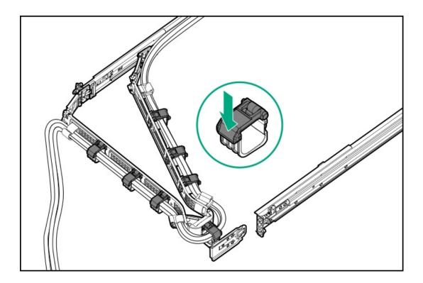
7. Align and install the elbow bracket.
