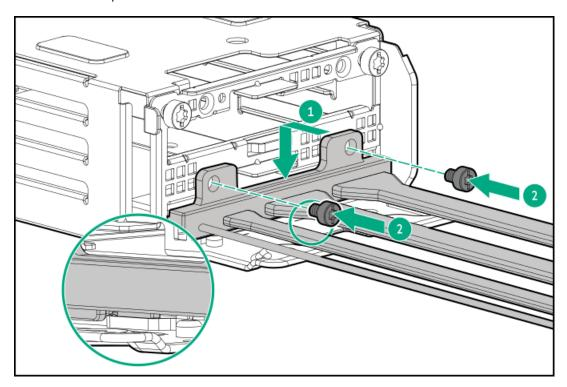
3. If you are not immediately installing the secondary front OCP NIC cable, install the other two screws on the bracket as spares.
