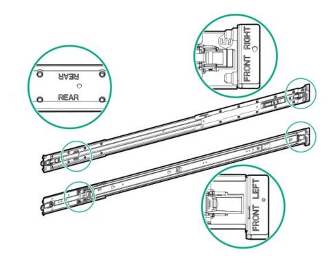
3. Extend the rack rails to align with the depth of the rack.
