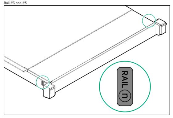
• Rail identifier stamps on the inner rail of the friction rack rail
