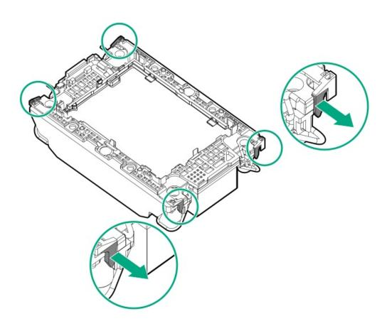
d. Lift the processor carrier away from the heatsink.
