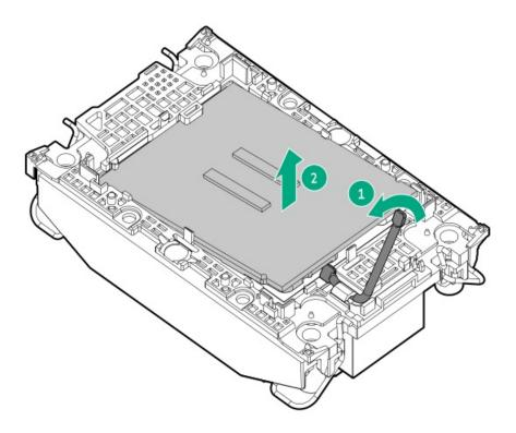
c. Starting from the pin 1 corner and moving in an opposite manner, disengage the processor carrier release tabs from the heatsink.
