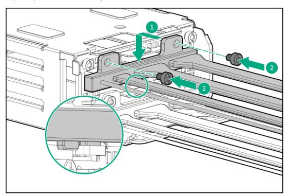
Installing the OCP NIC adapter in the E3.S cage
