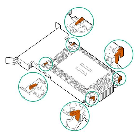
b. Verify that the pin 1 indicators on the processor and processor carrier are aligned.
