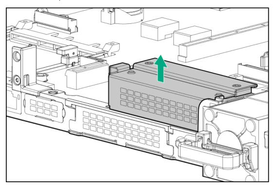
10. Using a T-15 Torx screwdriver, remove the rear riser support bracket.
