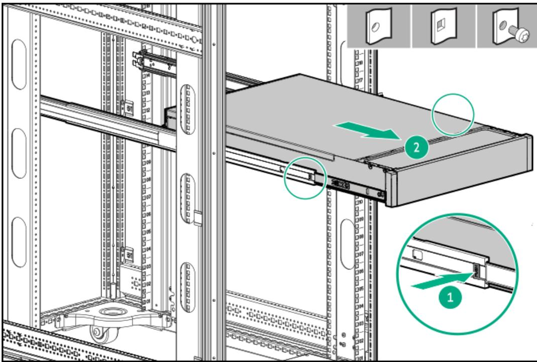
2. Unlock the spools from the locking tab and then remove the server.
