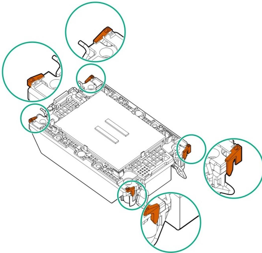
b. Verify that the pin 1 indicators on the processor and processor carrier are aligned.
