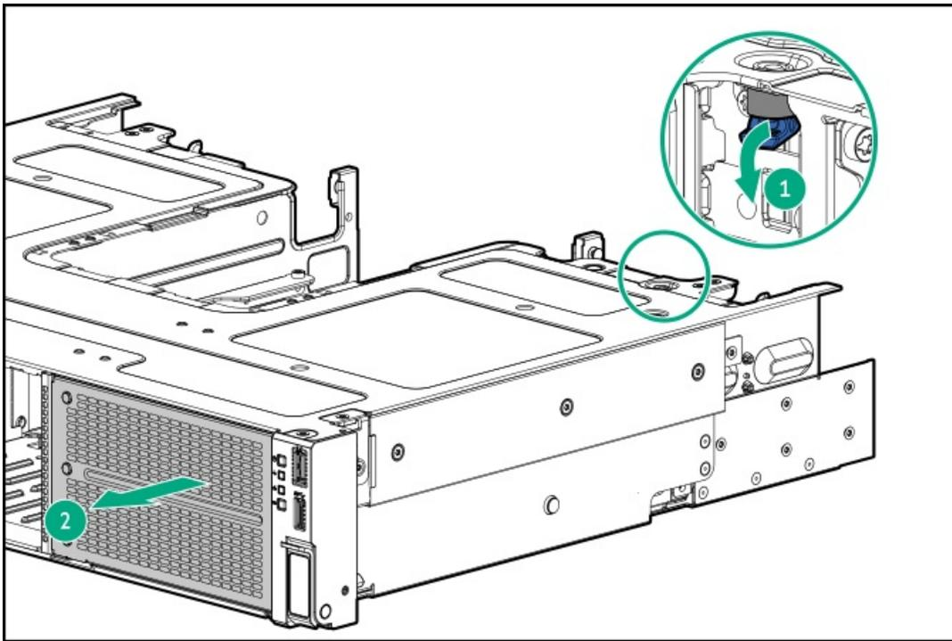
14. Remove the GPU riser cage cover.
