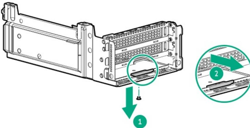
17. Install the boot device assembly on the secondary riser cage.
