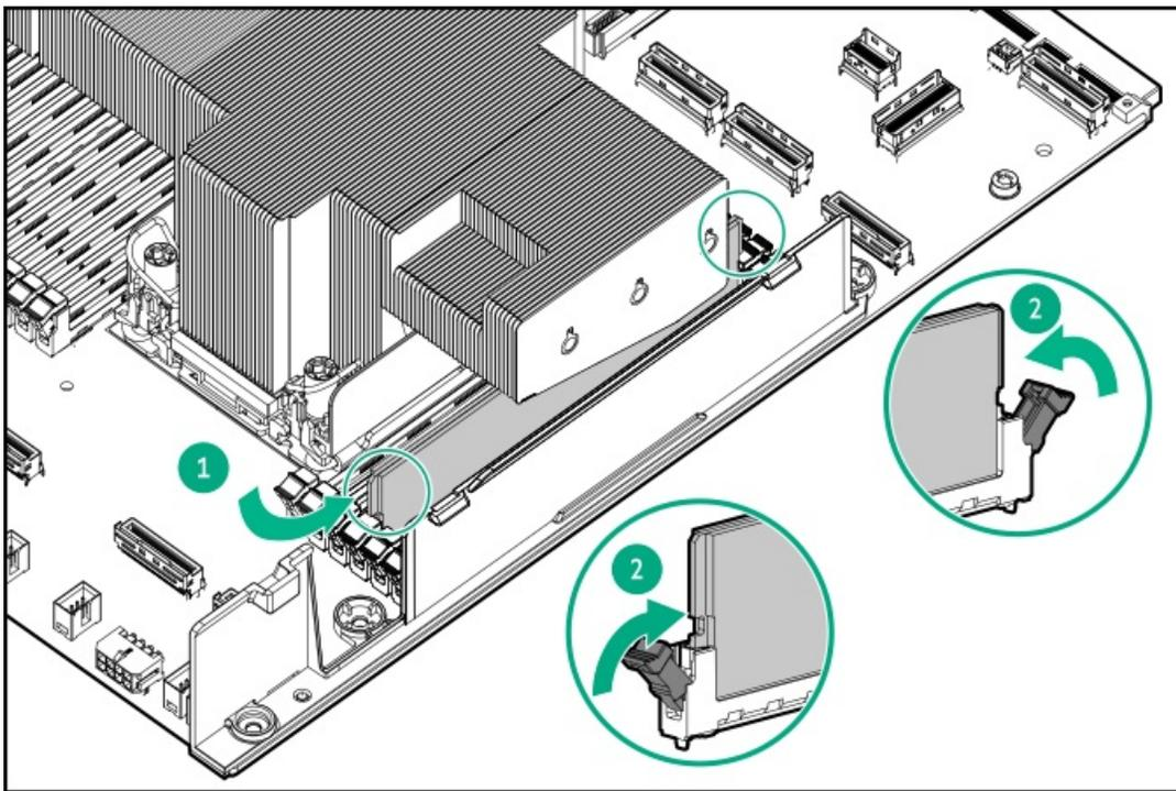
11. To install a DIMM with the standard heatsink installed:
