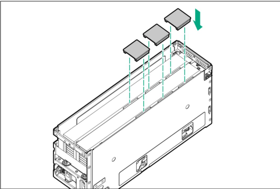
23. Install the GPU riser cage cover.
