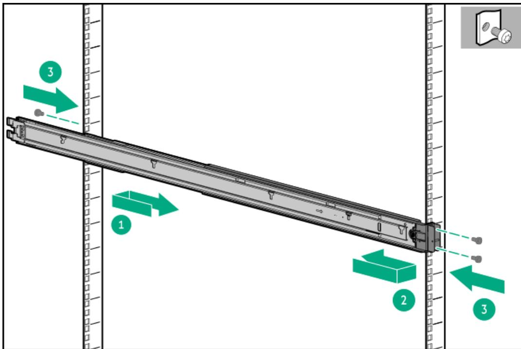
3. Fully extend the rails to the locked position.
