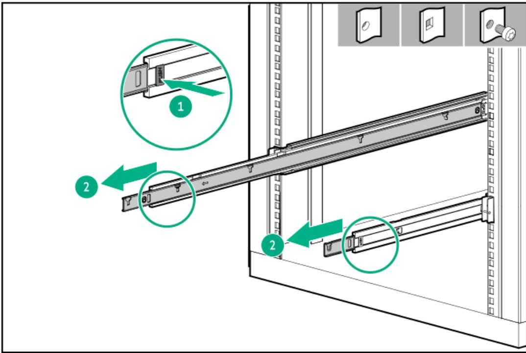
4. Verify that the rails are fully extended and the slots are aligned.
