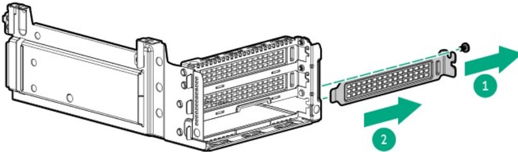
16. Remove the boot device cover from the secondary riser cage.
