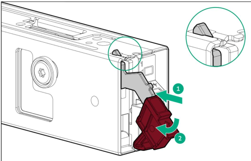
**Installing the boot device**
