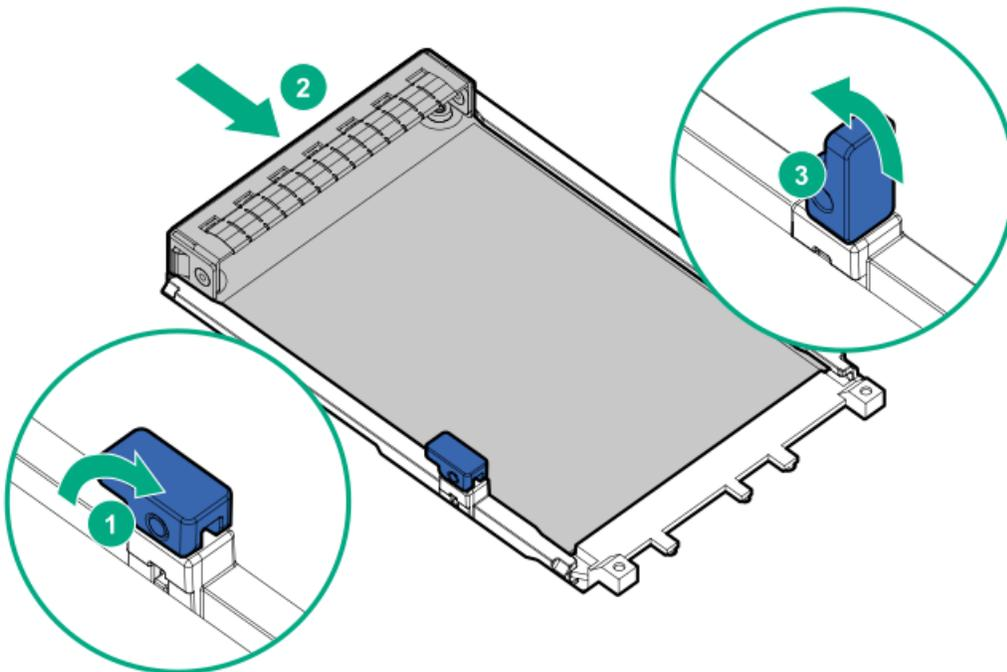
13. Install a riser cageInstall the riser cage.
