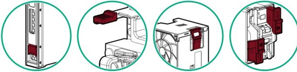
Hot-plug red indicates hot-pluggable components. These components can be removed and installed while the system is running, and doing so will not result in a system shutdown.
