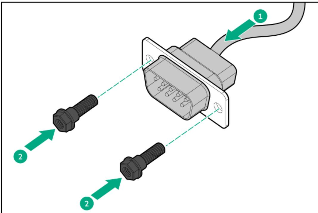
12. Connect the serial port cable to the system board.
