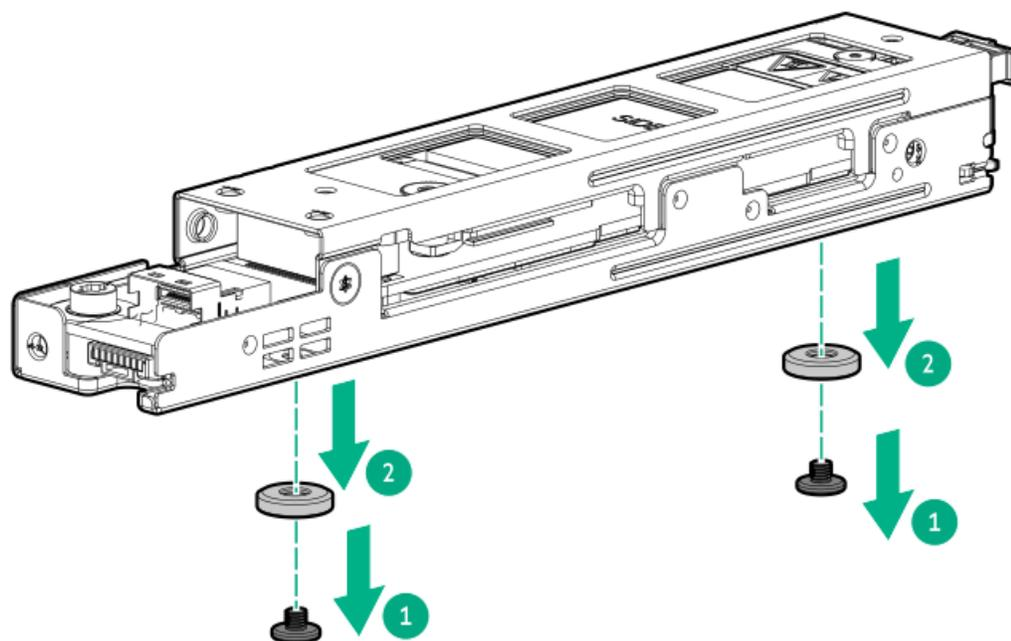
13. Install the boot device onto the bracket:
