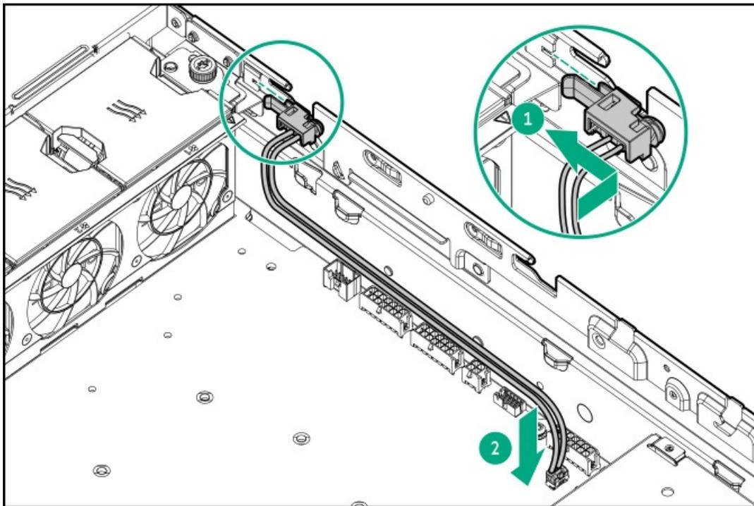
9. Connect the chassis intrusion detection switch cable to the system board .
