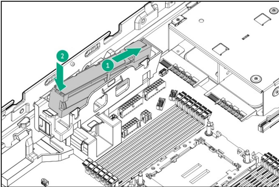
11. Connect the energy pack cable to the system board.
