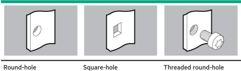
The illustrations used in this procedure show an icon on the upper right corner of the image. This icon indicates the type of mounting interface for which the action illustrated in the image is valid.
