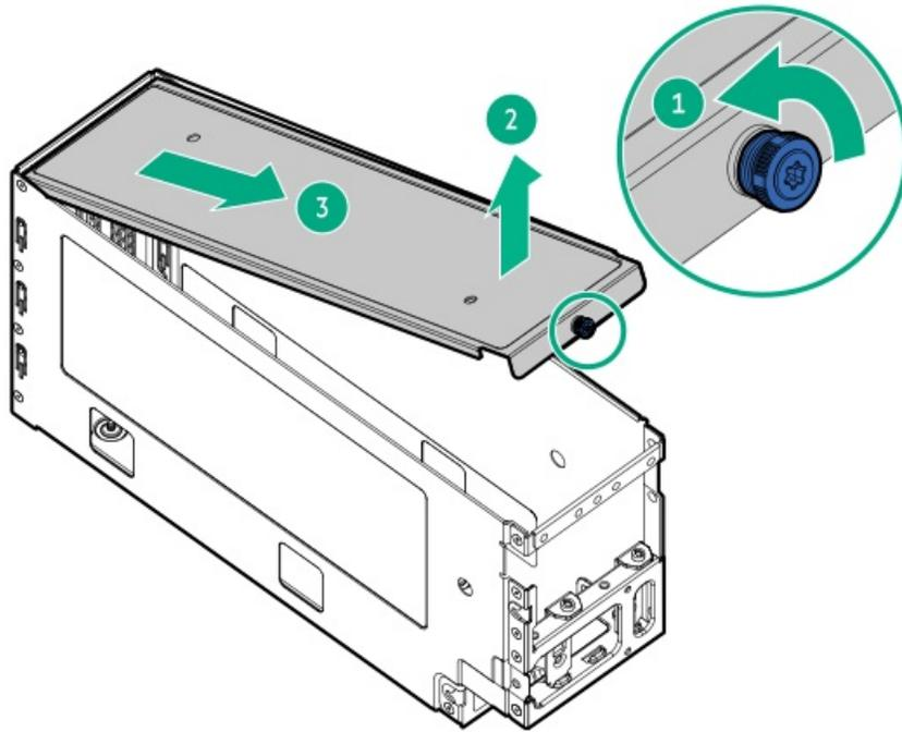
15. Remove the GPU riser slot brackets.
