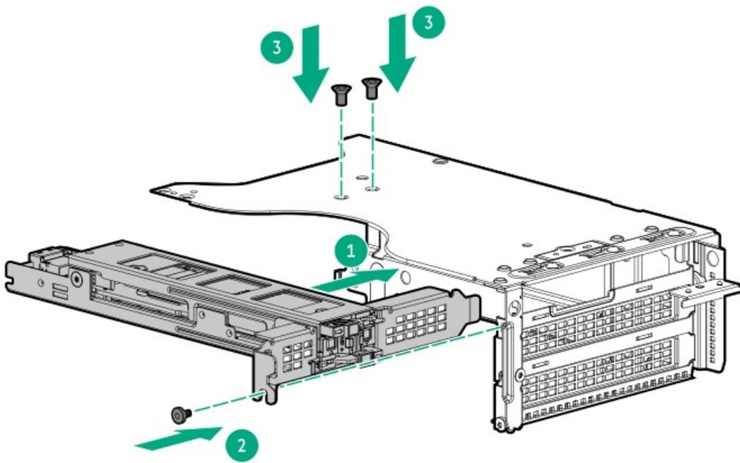
18. Install a riser cageInstall the riser cage.
