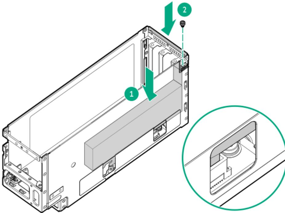
18. Install the GPU riser cage cover.
