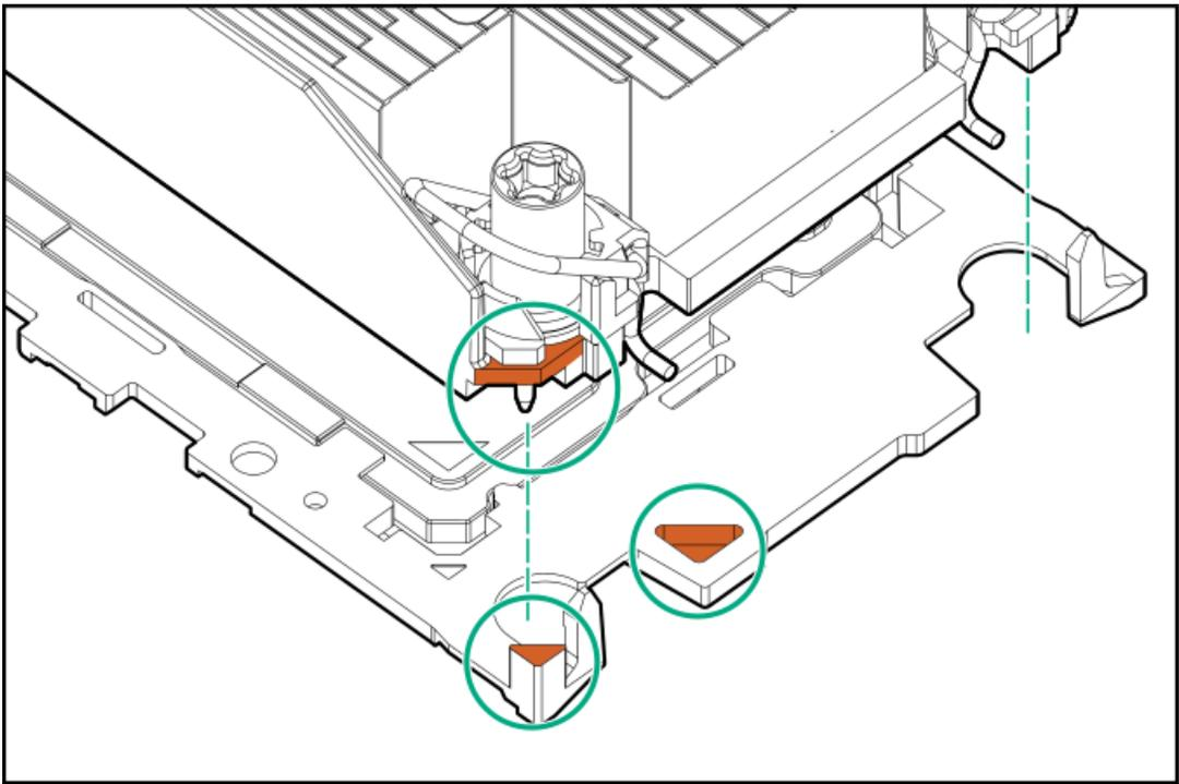
b. Lower the heatsink on the processor carrier until the carrier tabs snap into place. There will be an audible click to indicate that the heatsink is properly latched on the processor carrier.
