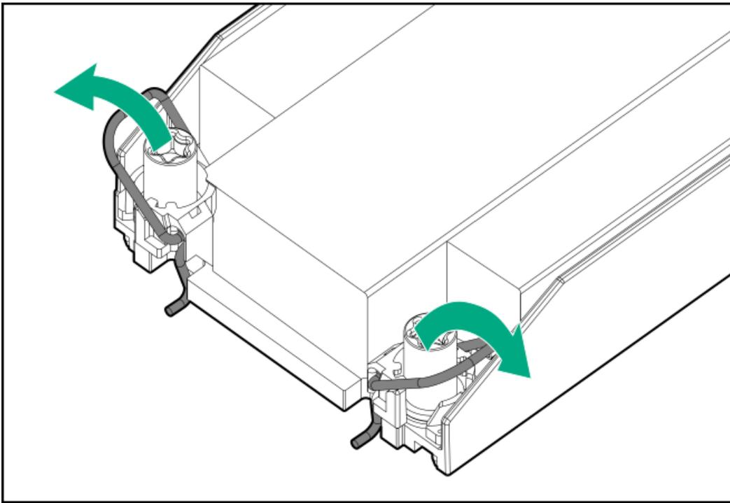
e. Tighten one pair of diagonally opposite heatsink screws, and then tighten the other pair of heatsink screws.
