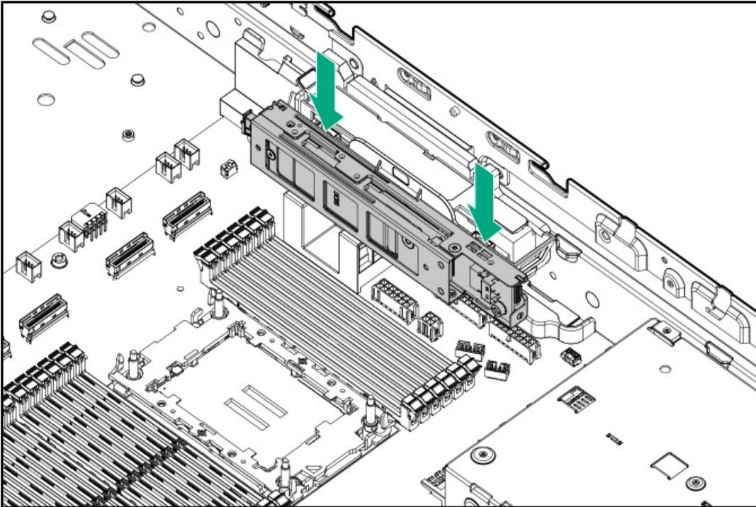
13. Connect the internal HPE NS204i Boot Device cables.
