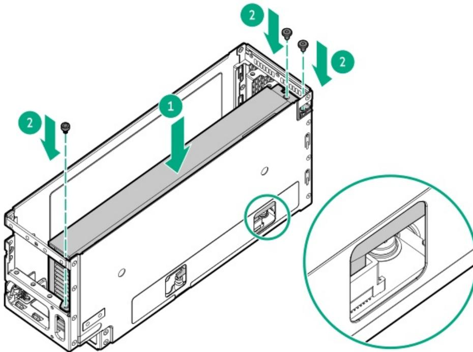
20. To install a second double-width GPU, do the following:
