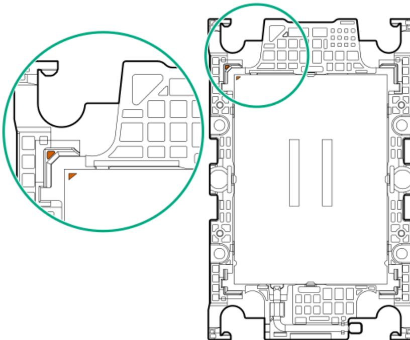
c. Verify that the processor is properly secured by the carrier snaps.
