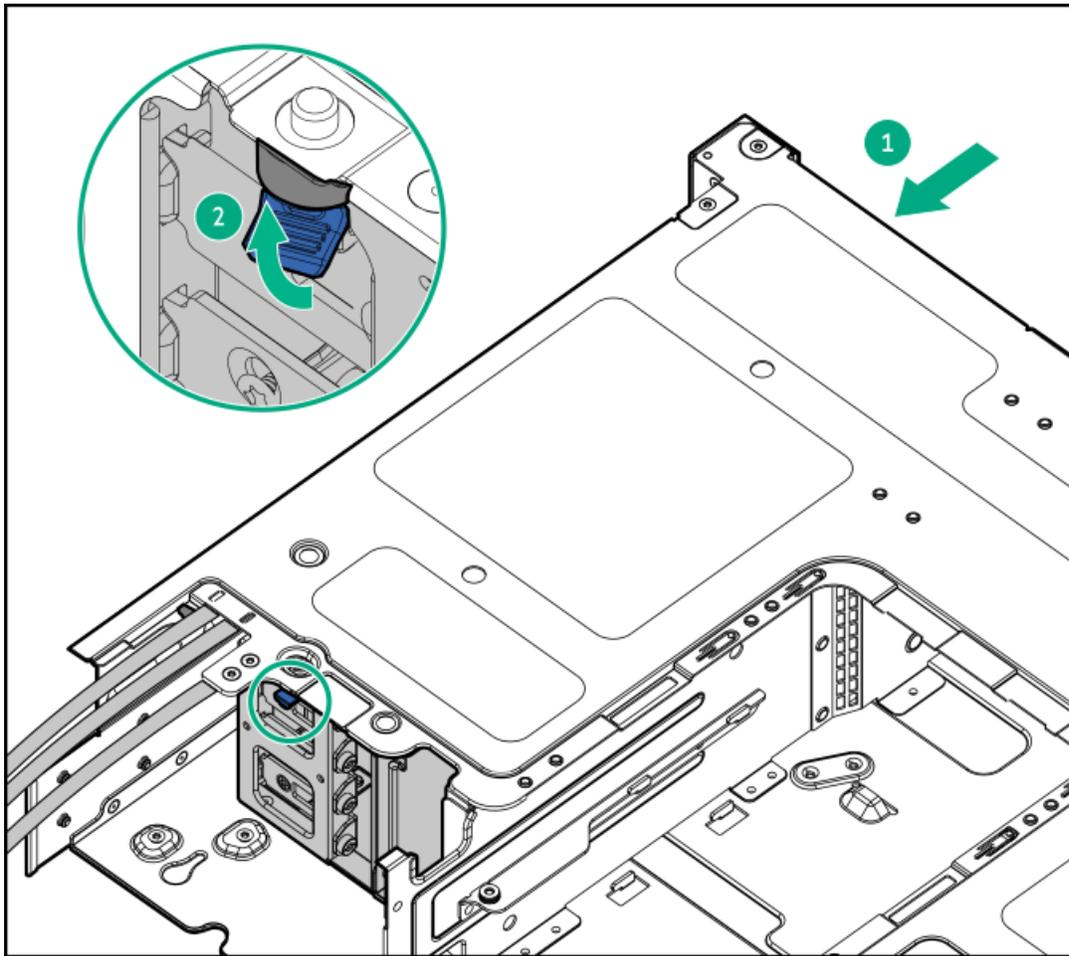
20. Connect the GPU riser cables to the system board.
