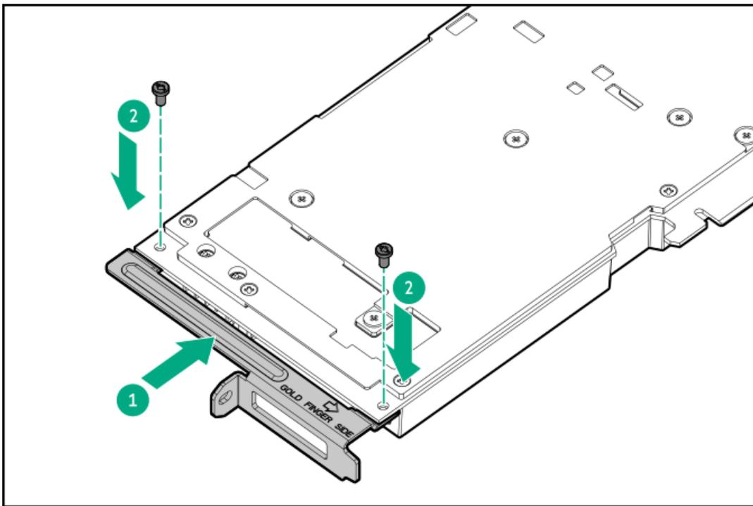
17. Install the single-width GPU in the riser, and then secure the screws.
