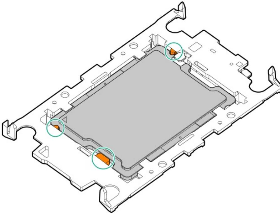
14. Attach the heatsink to the processor carrier:
