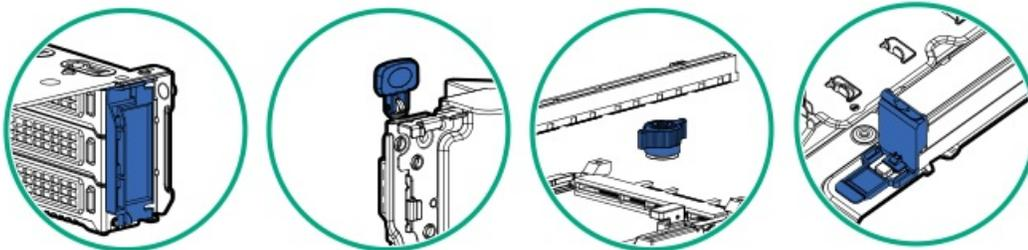
Touchpoint blue indicates cold-pluggable components. These components require a system shutdown. Failure to do so might result in system failure or data loss. Cold-pluggable components might also indicate touchpoints on non-electrical components.
