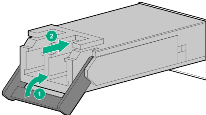
2. Remove the dust plug or protective cover from the transceiver.
