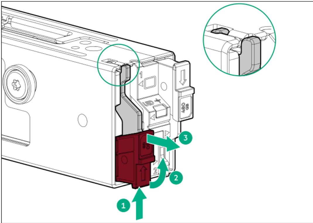
2. Install the SSD on the boot device carrier:
