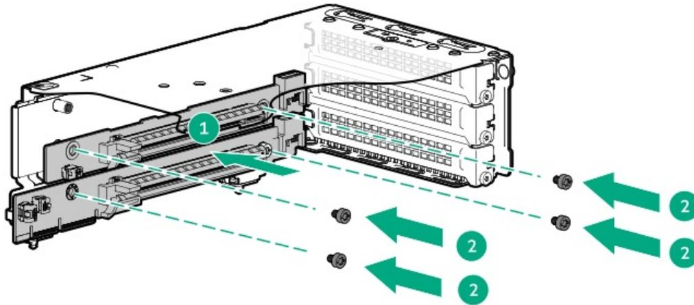
14. [Install a riser cage](#)Install the riser cage.
