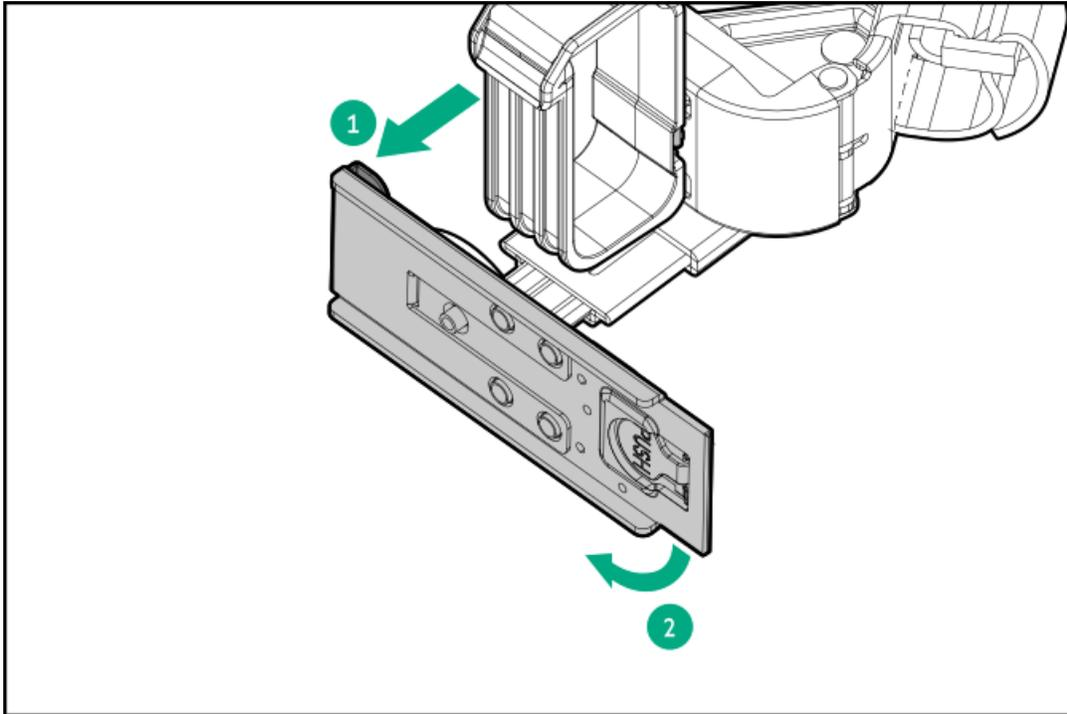
3. Connect the CMA hinged tabs and retention bracket to the rack rails:
