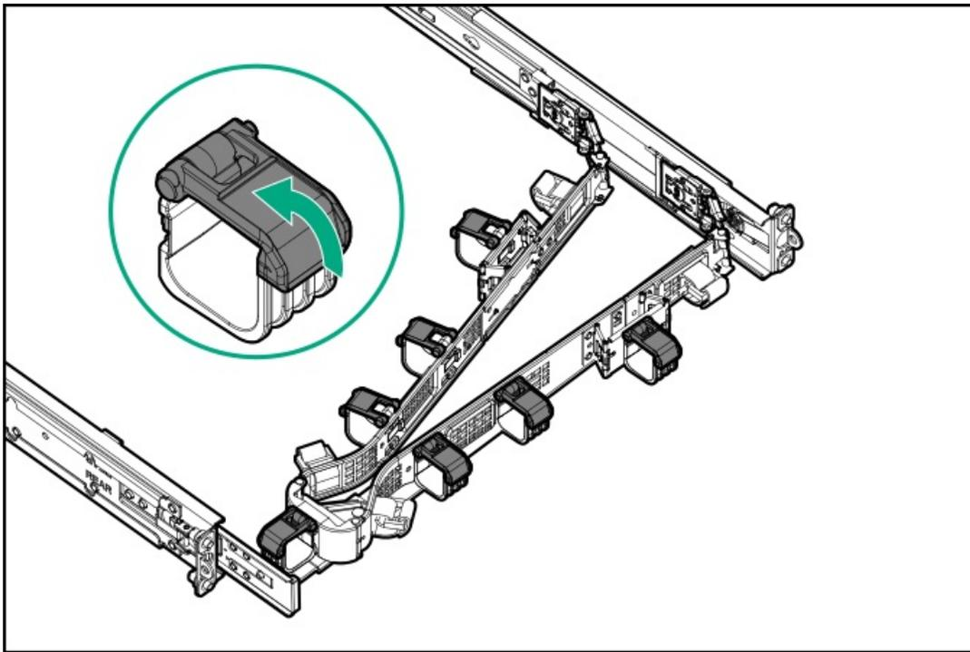
5. (Optional) If your CMA has cable straps for additional cable strain relief, unwrap the straps.
