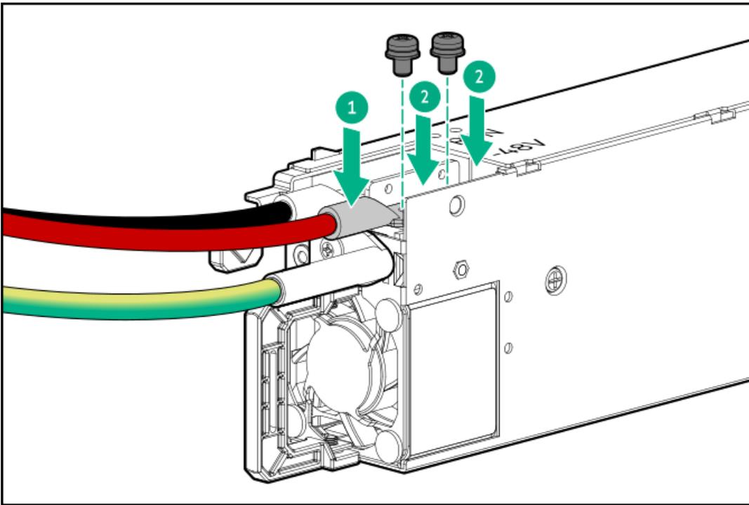
6. Install the protective cover on the DC power supply.
