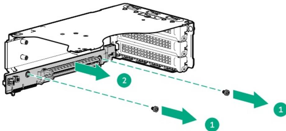
12. Connect the stacking riser to the base riser.
