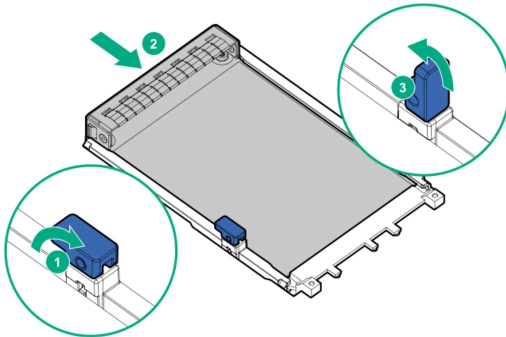
12. Install a riser cageInstall the riser cage.
