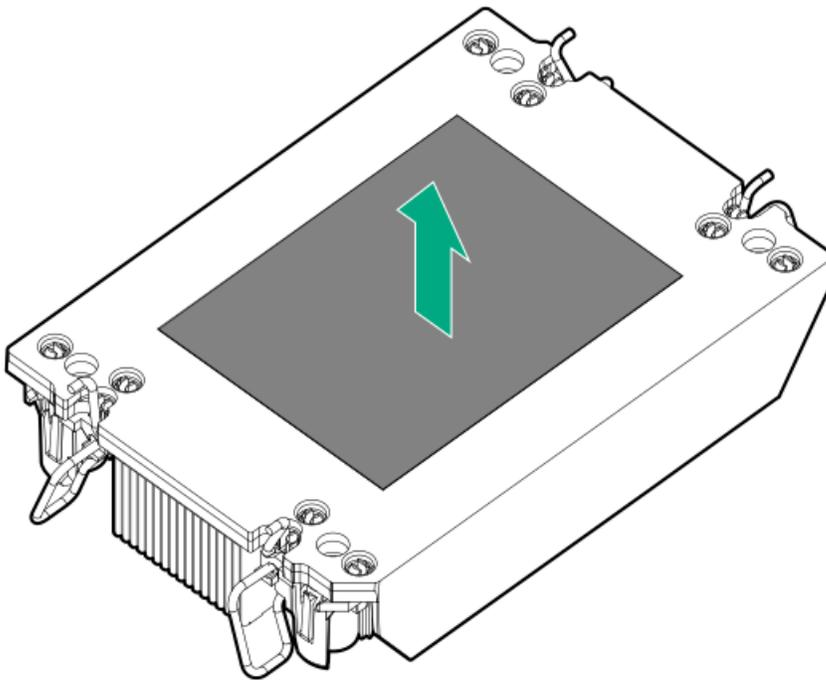
11. Set the anti-tilt wires to the unlocked position.
