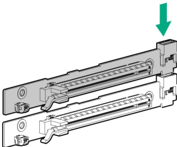
13. Install the riser on the riser cage:
