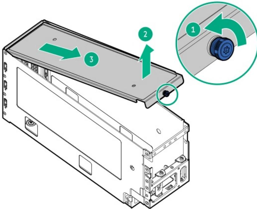
15. Remove the GPU riser slot brackets.
