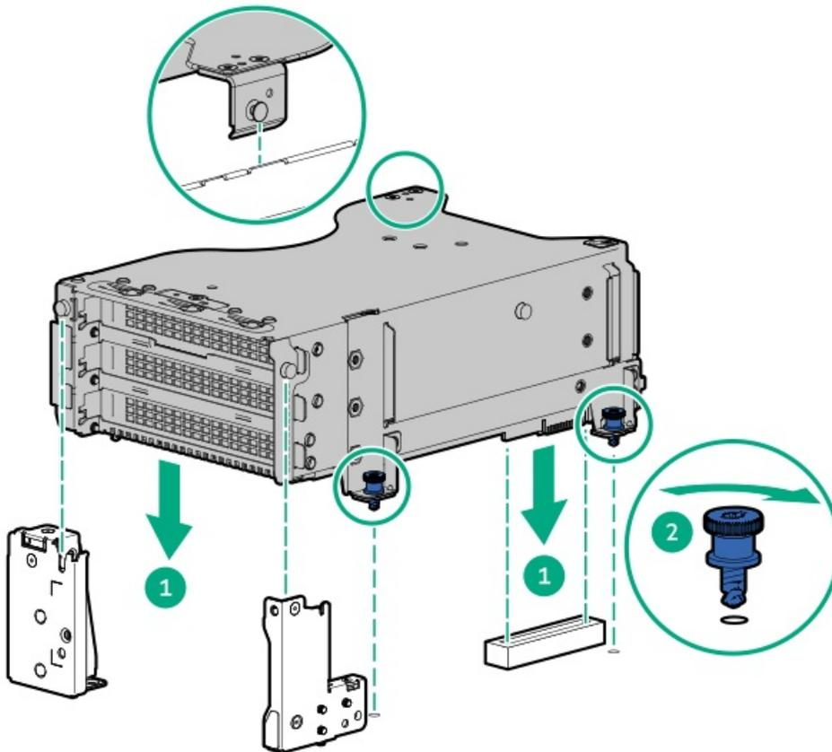
3. To install the secondary riser cage:
