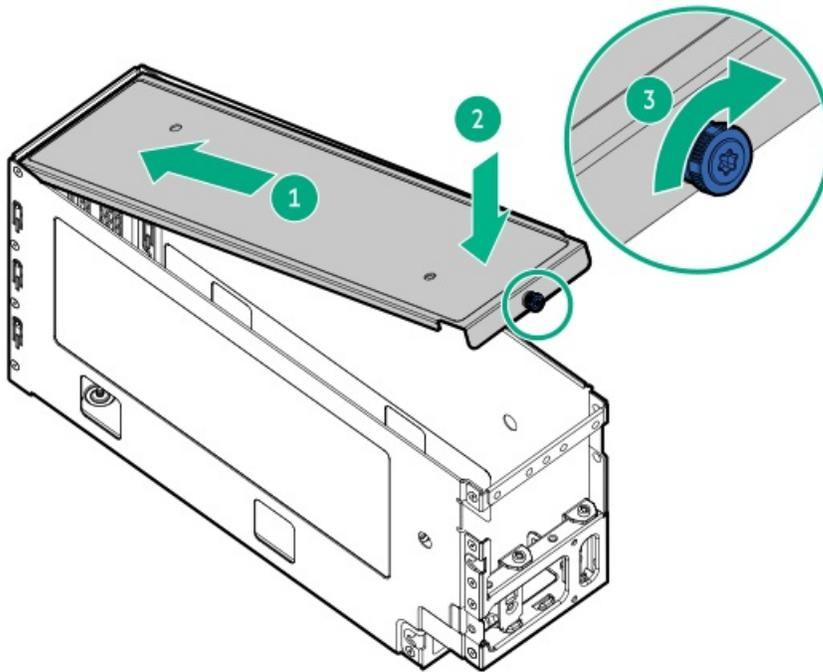
19. Install the GPU riser cage:
