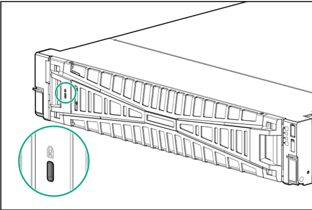
2. Press the bezel release latch, and then pivot the bezel open.
