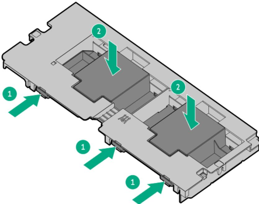
2. Install the air baffle.
