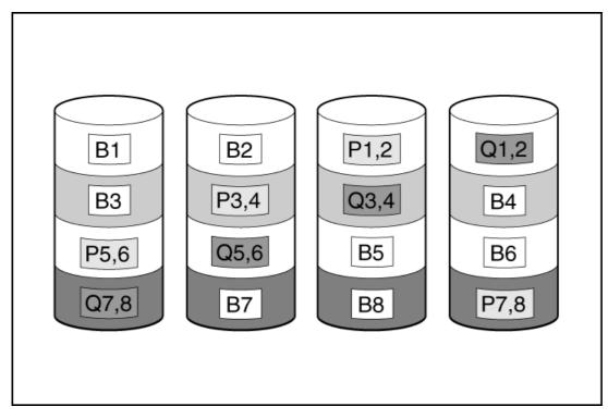
This method is most useful when data loss is unacceptable but cost is also an important factor. The probability that data loss will occur when an array is configured with RAID 6 (Advanced Data Guarding (ADG)) is less than it would be if it were configured with RAID 5.
