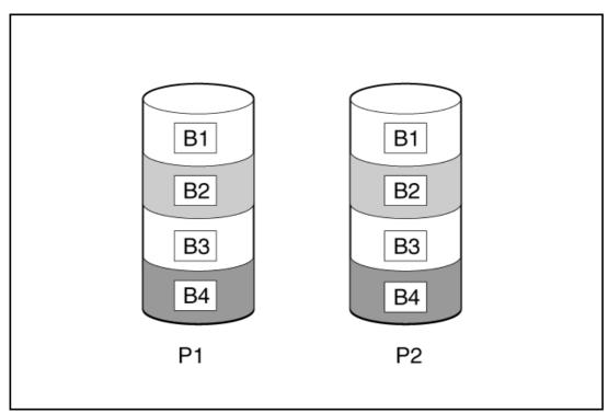
When the array has more than two physical drives, drives are mirrored in pairs, and the fault-tolerance method is known as RAID 1+0 or RAID 10. If a physical drive fails, the remaining drive in the mirrored pair can still provide all the necessary data. Several drives in the array can fail without incurring data loss, as long as no two failed drives belong to the same mirrored pair. The total drive count must increment by 2 drives. A minimum of four drives is required.
